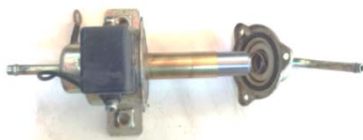
Fig 2. Test materials. Fuel electrical pumps.
